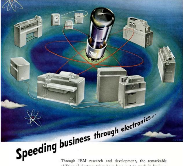
The IBM machines illustrated use electronic principles. Clockwise from the top, they are: Electric Time System, with Electronic Self-regulation; Alphabetical Collator; Statistical Machine; Card-programmed Calculator, including Calculating Punch; Punched Card Sorter. For descriptive literature, write to Dept. N.
